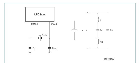
Fig 30. Oscillator modes and models: oscillation mode of operation and external crystal model used for  $C_{X1}/C_{X2}$  evaluation
