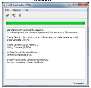
The bootloader code resides in the lower part of program memory (locations  $0-0\times0\,\mathrm{FFF}$ ). If the bootloader is mistakenly overwritten, it can be reprogrammed into the device through the programming connector, by programming the "HID Bootloader PIC18F67J94.hex" file into the device. This file can be found in the "HID bootloader" project directory.
